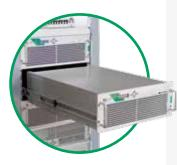
All PFG transmitters over 5kW can be equipped optionally with the hotplug system to instantly extract the amplifier modules with transmitter in full power.
