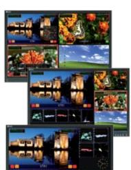
In addition to the standard quadsplit mode with four identical windows, there are different layouts available with several combinations of sizes and positions, along with the WFM tools.
